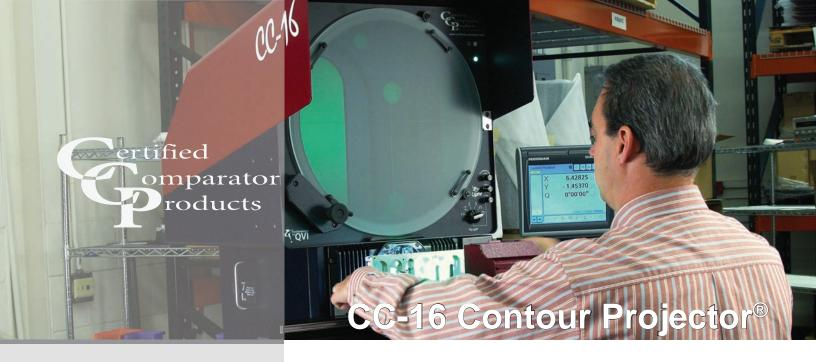
The CC-16 is a top quality optical comparator designed to meet the needs of today's manufacturers. The 16" diameter screen displays crisp, evenly illuminated images at every available magnification.
