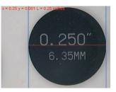
With calibrated overlays on the screen, the operator can compare a known dimension to the live image.
